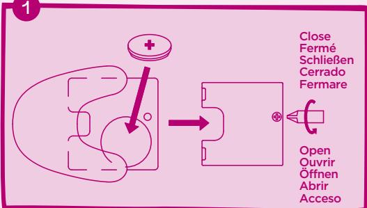
(EN): To replace batteries: Unscrew the battery cover and replace 1 x CR2032 size battery.
