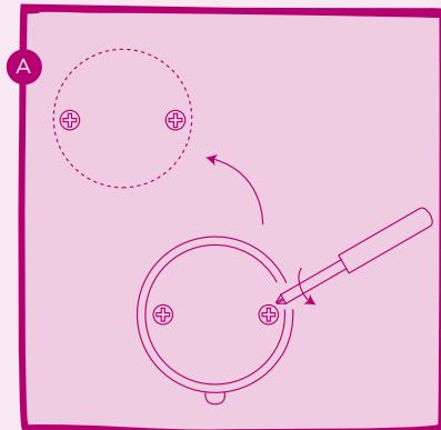
(EN): Open the battery cover with a screwdriver.
