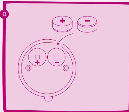
(EN): Install 2 x AG13 (L1154) batteries and follow the polarity orientation, as shown.
