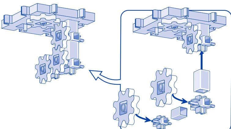
Continue to build by adding a pillar to the top of the six-way axle and attaching another six-way axle. Add a pillar to the side of a six-way axle to build horizontally.
