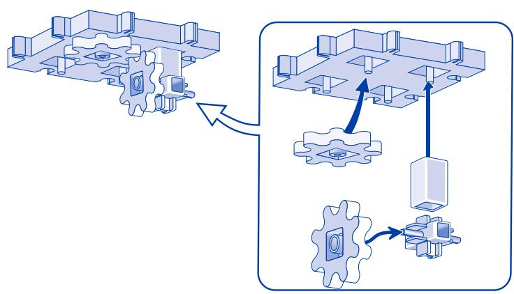
Begin in vertical structures by placing a pillar into the square hole on a base. Then, add a six-way axle and attach gears to the axle, making sure the "teeth" mesh at a right angle with the gear on the base. The gear on the axle should spin when you turn the gear on the base.
